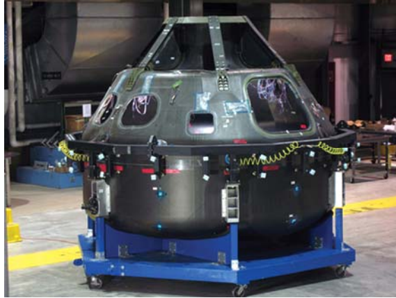
Image 2. The design and construction of the NASA Composite Crew Module (CCM) was optimized with the help of HyperSizer structural sizing and design analysis software. The module is pictured here with sensors attached in preparation for pressure testing. Photo courtesy of NASA
